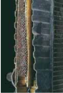
Dirty Transmission Cooler
